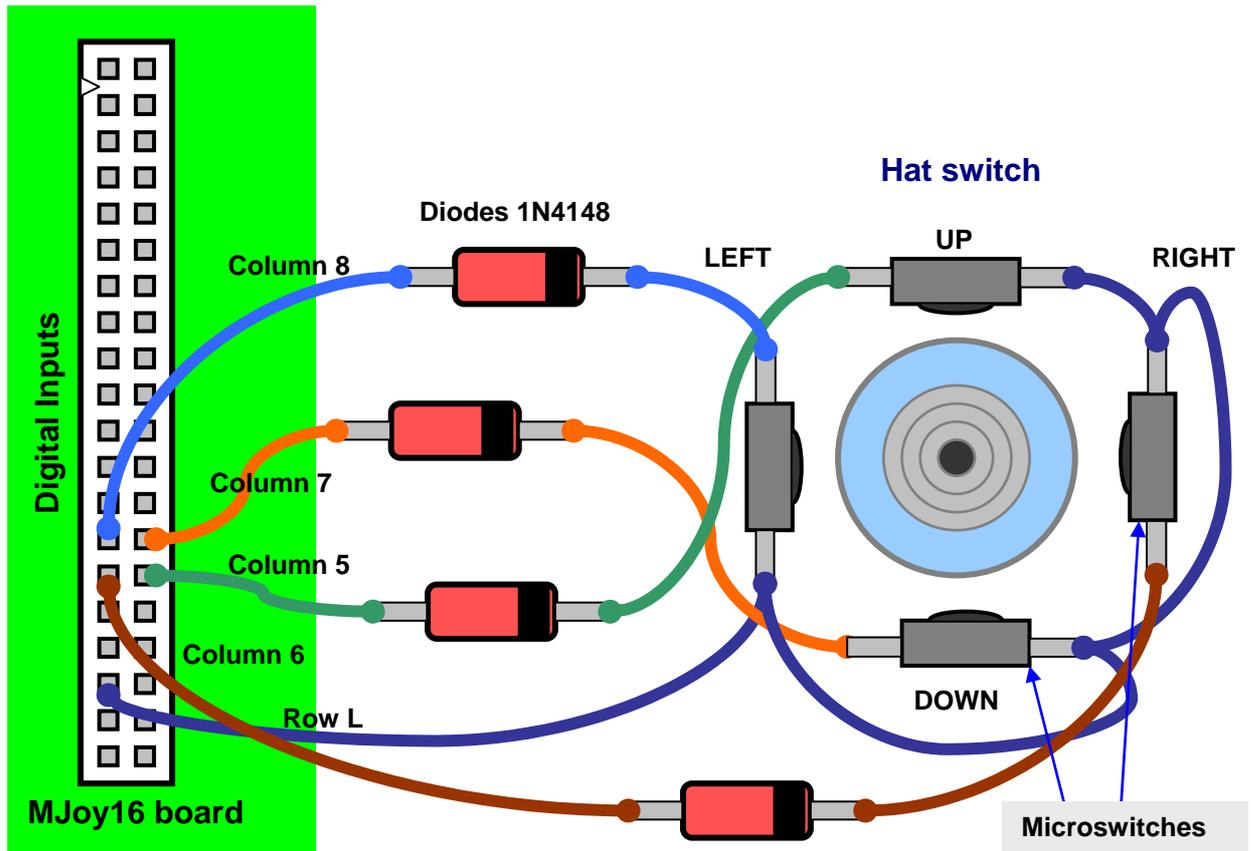
Below is a diagram showing how to wire hat switch to the Key Matrix board:
