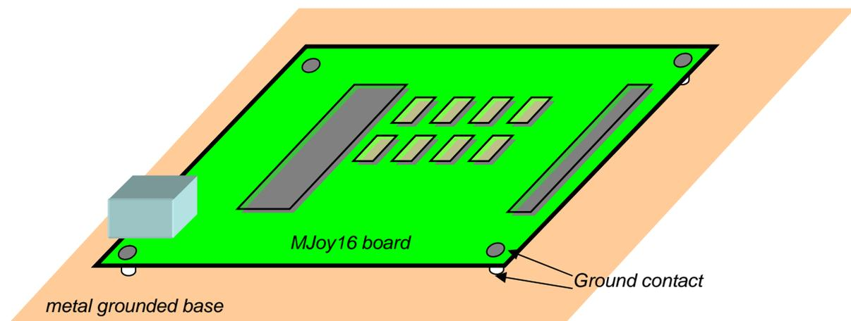
Generally your cockpit frame should be grounded to minimize possible interference. But some cockpit designs might have some power actuators installed. In these cases such power devices ground should be separated from signal ground and filtering measures installed if needed. MJoy16 board should be connected to signal ground plane.
