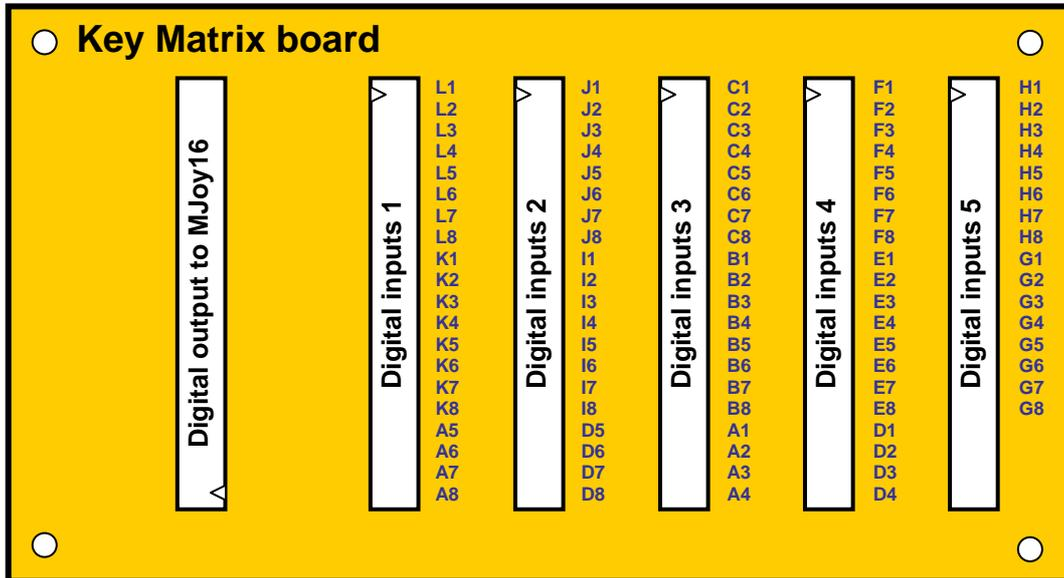
Key Matrix board consists of digital inputs and outputs.
