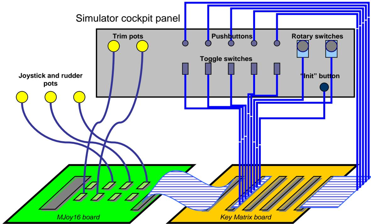
In this layout all wires can be laid out as a bundle along the edges of the panel. This provides easy maintenance access to all buttons and switches.
