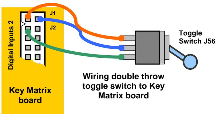
Please note that in above diagram wire from pin 4 (next to green wire) of digital inputs was not used. This is because pins 2 and 4 are already interconnected on the connector so extra 4<sup>th</sup> wire is not needed.
