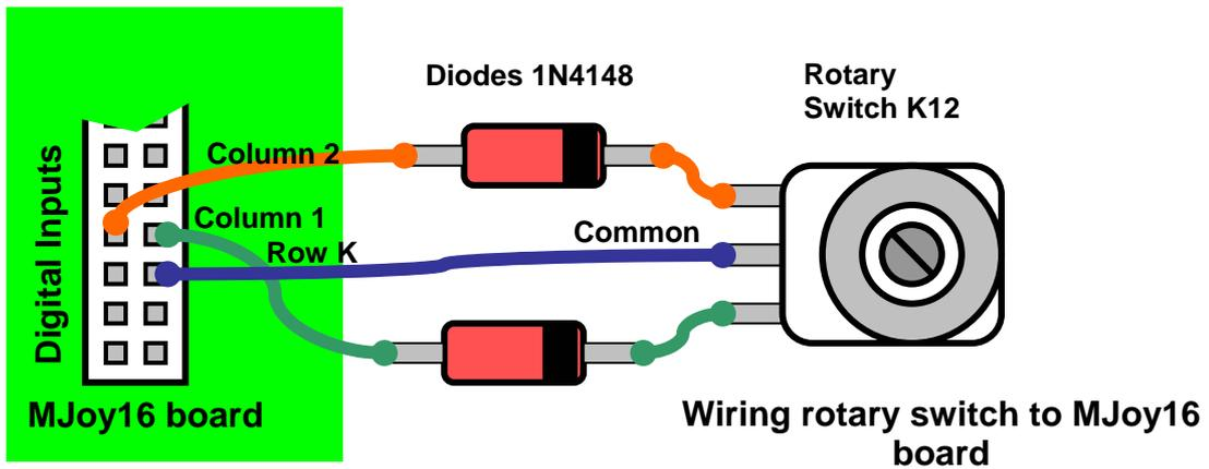
If you wire rotary switch through Key Matrix board you should follow the example below:
