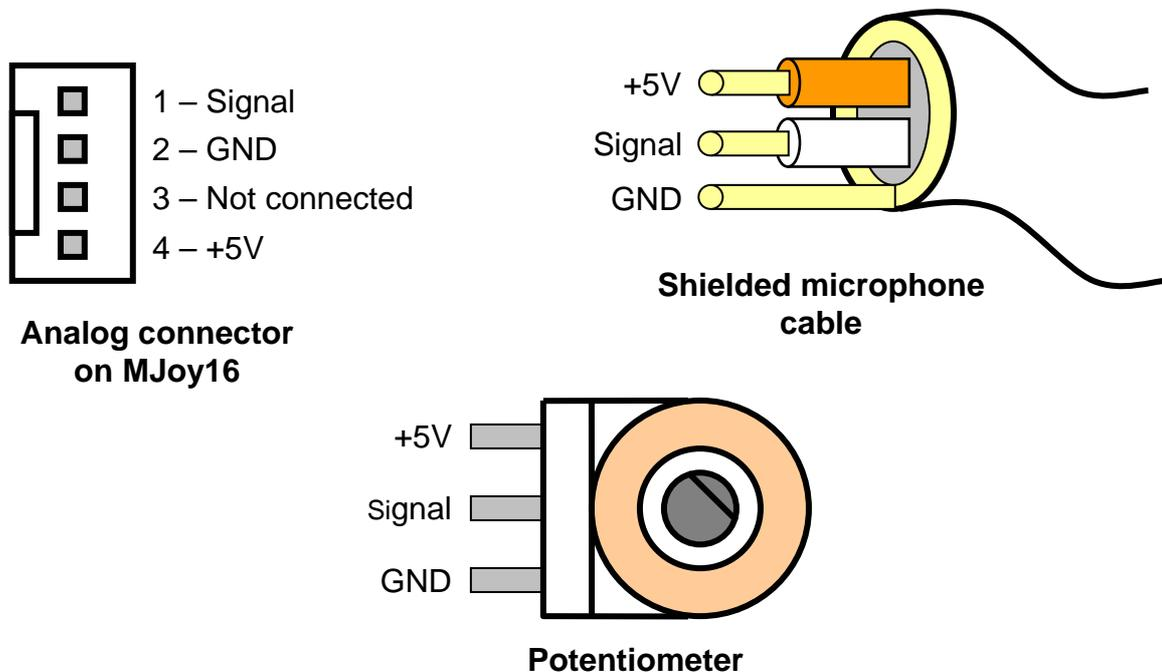
It is recommended to connect potentiometer using shielded cable as short as possible.
