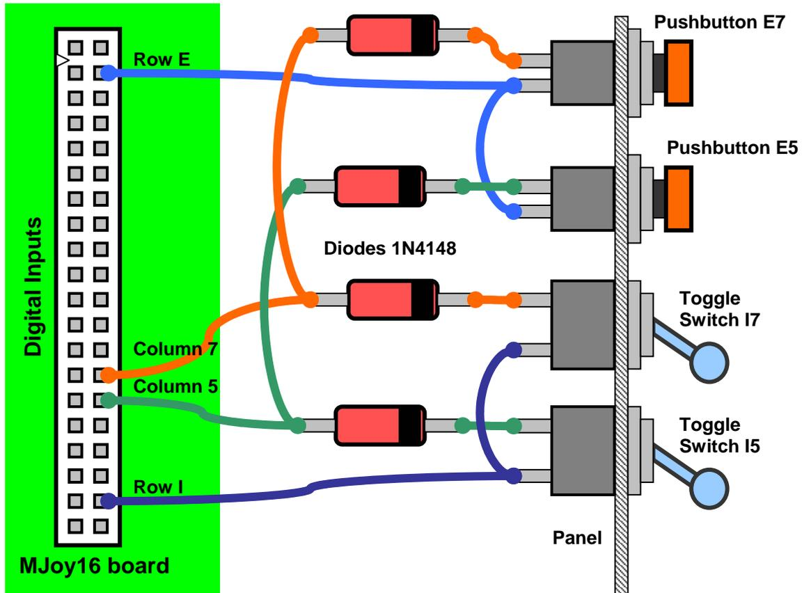
It can be seen that a lot of soldering is made directly to the panel and there are wires that are going from one control or diode to another. With more controls this complexity increases even more. Different types of digital controls are wired in slightly different ways. Exact wiring of them will be described further in this chapter. Key Matrix greatly simplifies wiring and possible rewiring of the panel.
