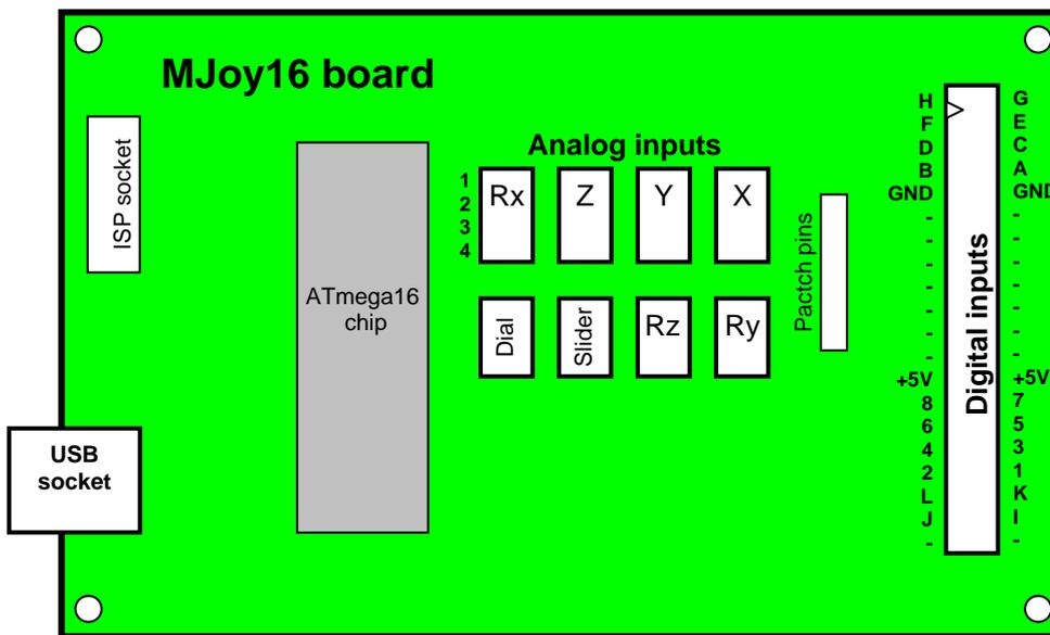
The main connectors on MJoy16 board are USB socket, Analogue Inputs and Digital inputs. The board USB socket takes a B type USB cable which connects it to host computer.
