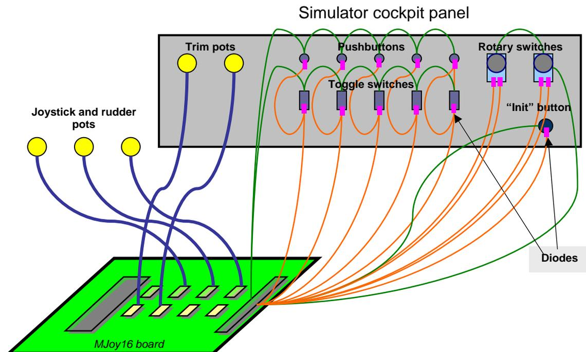
As you see in the diagram above you must form a wiring matrix of all buttons and switches directly on the panel plus soldering the diodes to each digital control.
