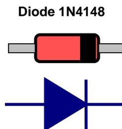
This band colour may be other colour depending on typical body colour of the diode. Other types may have different marking convention.
