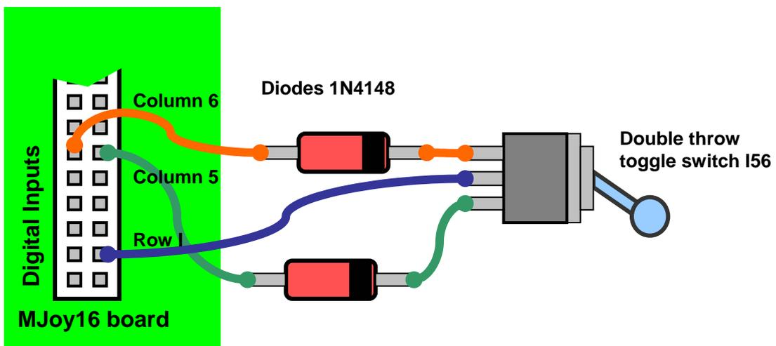
Below is an example of a double throw toggle switch wiring to the Key Matrix board
